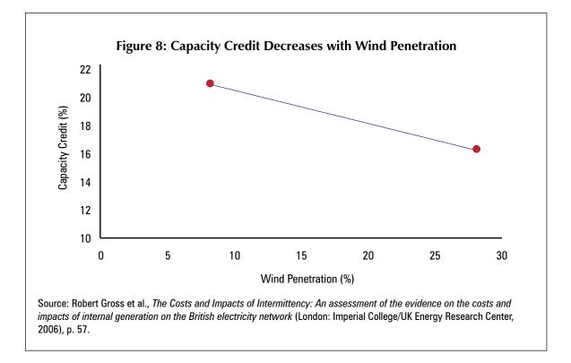
Figure 8 from Gross et al. shows that capacity credit decreases as wind penetration increases.<sup>21</sup> This is because at high wind penetrations, additional reserves are required to ensure the same level of grid reliability. Gross et al. show further that the crossover between high and low capacity credit occurs in the neighborhood of 20% wind penetration.<sup>22</sup>
